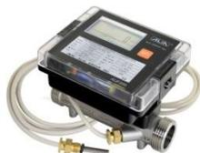
**AUF200 Series** measure flow or energy of water running in heating/cooling pipe by temperature sensor based on ultrasonic flowmeter. It's simple, easy to install and battery powered, no need of external power. It can display flow rate, total flow, total heat, total cool, heat power and supply/return temperature etc..
