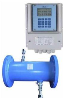
**AUF760 series** is a fixed mounted, transit-time ultrasonic flowmeter. It features factory mounted transducers that allow it to be flow lab calibrated reducing or eliminating the random or bias error that can be present in clamp-on style transducer mounting. The meter ensures an accurate, non-invasive measurement of clean homogeneous liquids process.
