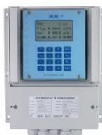
**AUF750 series** is a fixed mounted, transit-time ultrasonic flowmeter. It features clamp-on style transducers for non-invasive measurement of clean homogeneous liquid processes. This user friendly microprocessor based, field programmable flowmeter ensures that the flow of existing processes can be performed without interrupting the flow and has very low installation costs.
