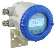
The **Aliamag AMC3200 series** converter is a microprocessor based intelligent transmitter that can be paired with any of the Alia AMF series sensors. The unit features multiple display parameters including flow rate, flow total, diagnostics, programming and troubleshooting. **It's equipped with bluetooth, HART and Modbus communication functions.**
