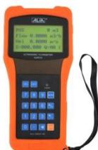
**AUF610 series** is a portable transit-time ultrasonic flowmeter with clamp-on transducers for non-invasive liquid measurement. Based on microprocessor and programmable flow measurement techniques the process flow can be accurately measured without interrupting the flow and with low installation costs. Transducers suitable for pipe sizes from 15 to 6000 mm , **high temperature transducers are available (Max. temperature 160°C )**
